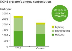
The calculation is based an elevator speed of 1.6 m/s, a load of 1000 kg, 200,000 starts/year, a travel height of 45 m and 15 floors
